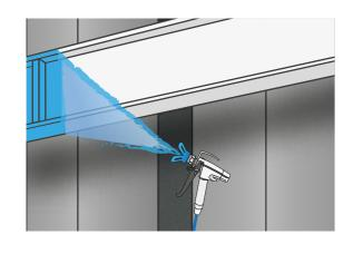
3. Hard to reach surfaces can be coated using the airless spray gun accessories, e.g. the extension tube and the linking nozzles.
