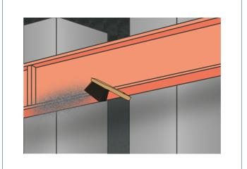
Alternatively, the steel can be coated by using a brush, roller or compressed air (PYRO-SAFE FLAMMOPLAST SP-A2 nozzle bore ≥ 3.5 mm, PYRO-SAFE Dekorlack SP 2 top coat nozzle bore 1.5 - 2.0 mm).
