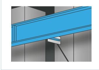
2. Once the coating has completely dried out, use a dry film thickness measuring device to determine the thickness of the dry film.
