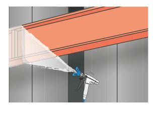
4. Hard to reach surfaces can be coated using the airless spray gun accessories, e.g. the extension tube and the linking nozzles.
